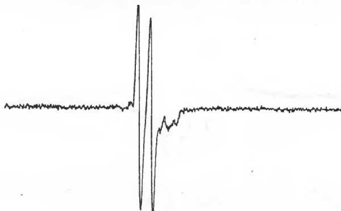
Fig. 5. EPR spectrum of a PPG + Na_2CO_3 + Ascorbate 1:1:1 mixture (3.3 mM) in the presence of the O_2 . A typical doublet of ascorbyl radical. Range: 336.5–334 mT. Gain: 2 \times 10^4 . Time constant: 20.48 ms, modulation amplitude: 1.013 G
