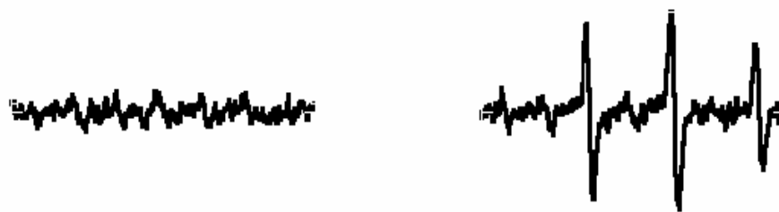
Fig. 2 : EPR spectrum of 1.5 \times 10^7 NIH/ml suspension in PBS + 18 mM DMPO (a) NO illumination (b) with 168s illumination while measurements. Measurement parameters: time constant 655 ms; resolution: 2048 points; modulation amplitude 1G; modulation frequency 100 KHz; conversion time 82 ms; gain 2 \times 10^5 ; power 20 mW.
