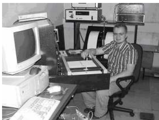
Fig. 5. An X-band (9.3 GHz) EPR spectrometer of RADIOPAN Firm (Poznań) with Rapid Scan Unit of JAGMAR Firm (Kraków).
