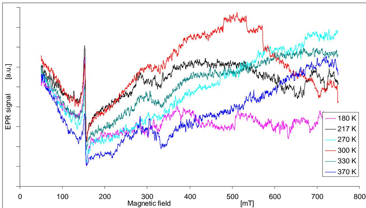
Fig. 4. The EPR spectra of mullites 0,012 at different temperatures.
