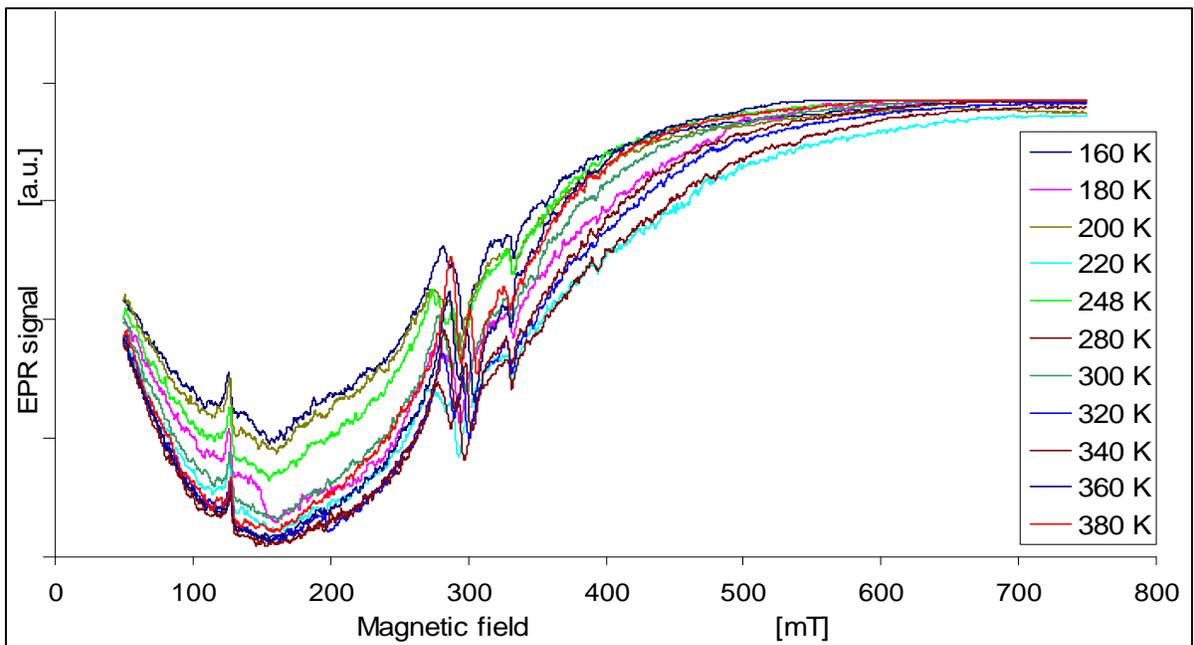
Fig. 2. The EPR spectra of  $\text{Al}_2\text{O}_3$  powder sample #325 at different temperatures.
