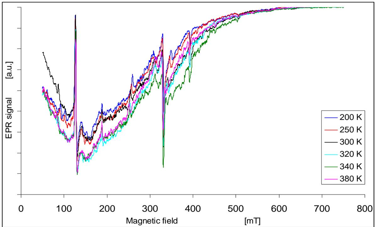
Fig.1. The EPR spectra of  $\text{Al}_2\text{O}_3$  powder sample #200 at different temperatures.
