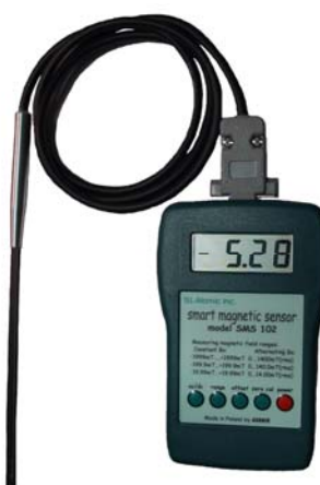
Fig. 10. Portable, Hall-Effect magnetic field meter
