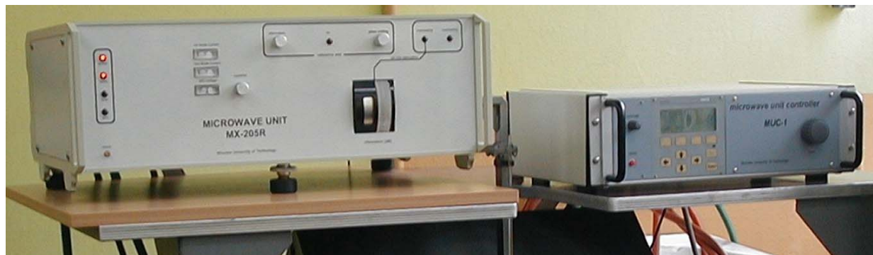
Fig. 8. X-Band microwave unit (older design)
