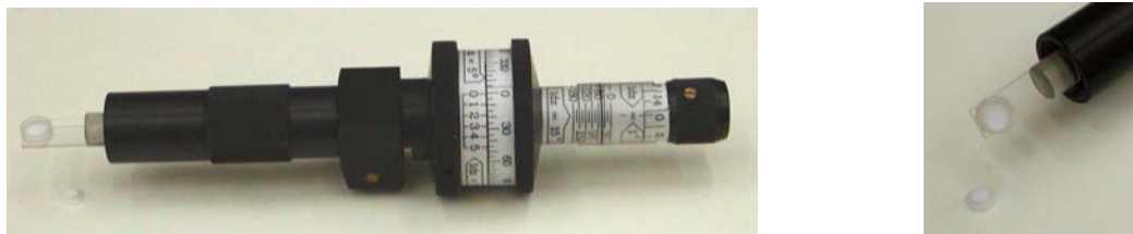
Fig. 7. X-Band two axis goniometer
