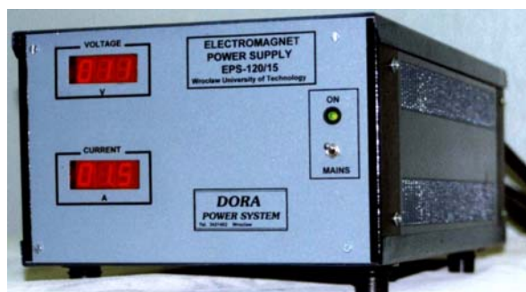
Fig. 9. High Efficiency Electromagnet Power Supply.
