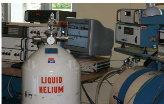
Fig.7. Electron Paramagnetic Resonance (EPR) spectrometer from JEOL 1967 (top), and from "Radiopan" 1982 (bottom).
